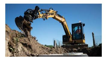
you could select a pin on top and an S-type bottom. The integrated grapple is only compatible when the TRS has the S-type lower interface.
