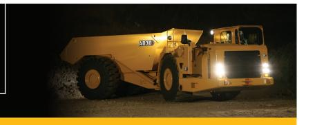
30 000 kg / 66,139 lb NOMINAL PAYLOAD CAPACITY 11.3-17.5 m<sup>3</sup> / 14.8-22.9 yd<sup>3</sup> BODY CAPACITIES
