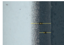
The depth of hardening on the stem face does not conform to specification, and the hardness of the grey market part is 25% lower, which will lead to increased wear.
