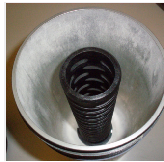
"Coreless" Element Removed from Housing
