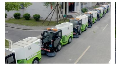
The RG-8240 offers a unique combination of features including an articulated, air-conditioned panoramic glass cab, a stainless steel collection bin, and a 'ballest-less' brush system that increases cleaning efficiency and extends brush life. Key functions including the walking drive, steering system, fan drive, brush drive and dust bin lift all use advanced hydraulic technologies.
