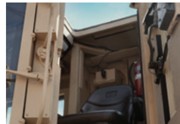
Emergency egress hatch.
