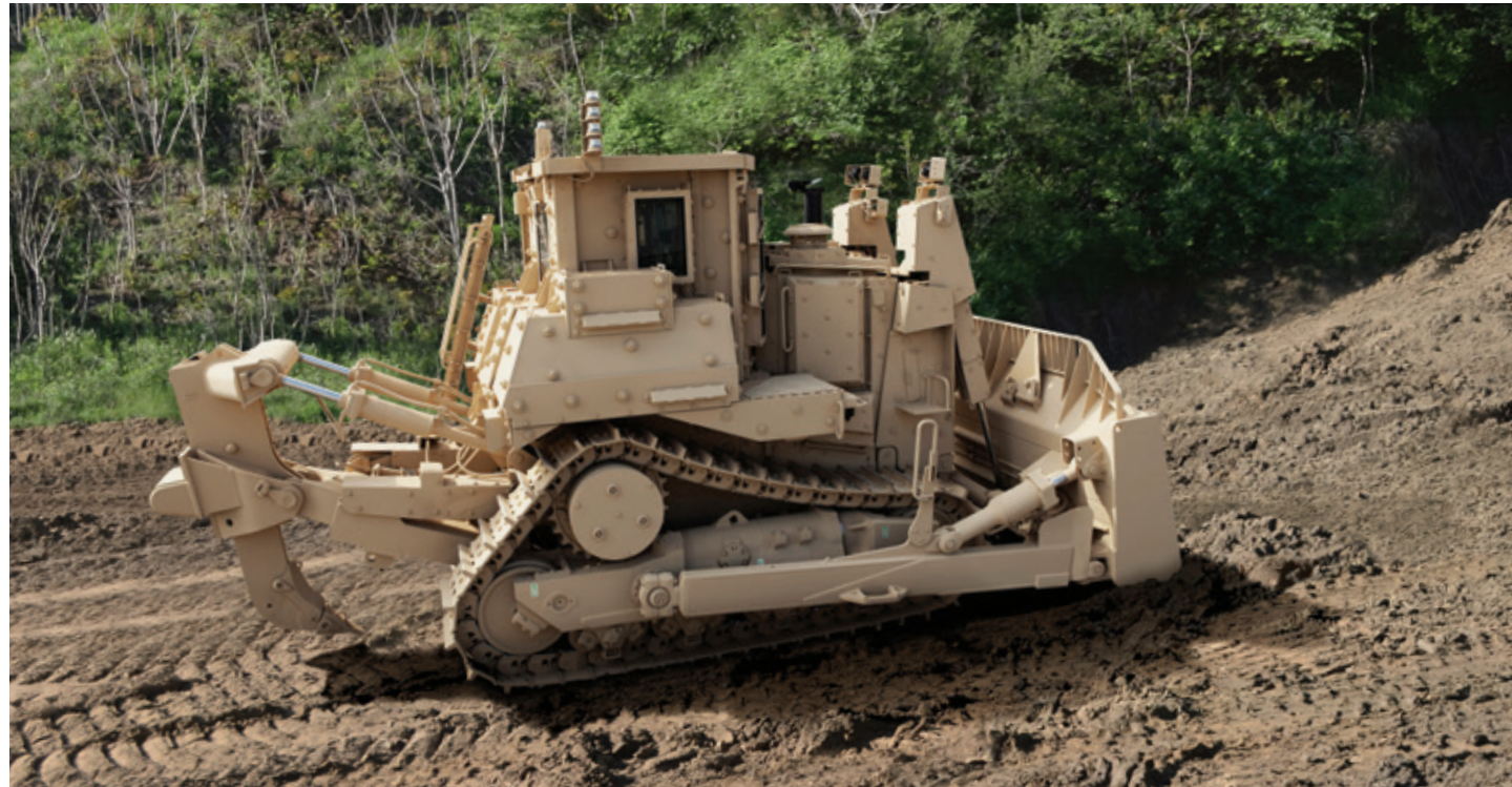
D9 fully armored with Crew Protection Kit (CPK) and Machine Armor Protection (MAP).
