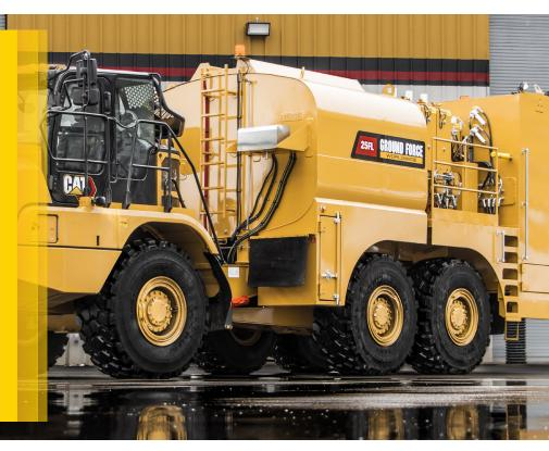
The rigid frame fuel and lube trucks are based on Cat Off-Highway Truck Bare Chassis ranging from models 770 to 793. Diesel fuel capacities range from 4,000 to 25,000 gallons (15 141 to 94 635 liters) and total oil and coolant capacities range from 1,000 to 8,000 gallons (3785 to 30 283 liters).
