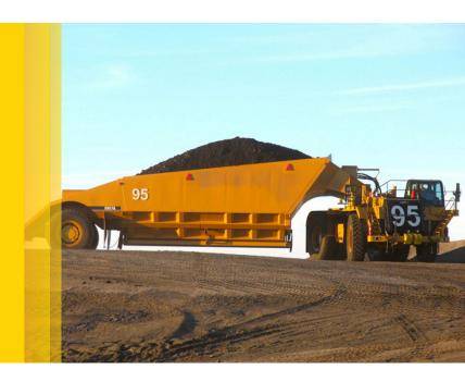
The simple and rugged gooseneck ball hitch design includes the components necessary to convert the truck chassis into a tow vehicle - including the hitch system, deck, fender, hydraulic system and brake control software. Mega trailers are equipped with suspended trailing axles utilizing Cat truck suspensions and wheel groups, including oil-cooled brakes and Cat brake control system components.
