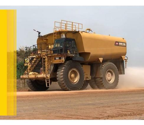
The rigid frame water trucks are based on Cat Off-Highway Truck Bare Chassis ranging from models 770 to 793. Capacities range from 9,000 to 52,000 gallons (34 068 to 196 841 liters).
