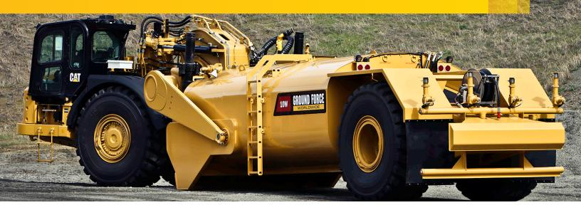
The water pull trucks are available based on the Cat 613 through 637 Wheel Tractor-Scraper. Capacities range from 5,000 to 12,000 gallons (18 927 to 45 242 liters).
