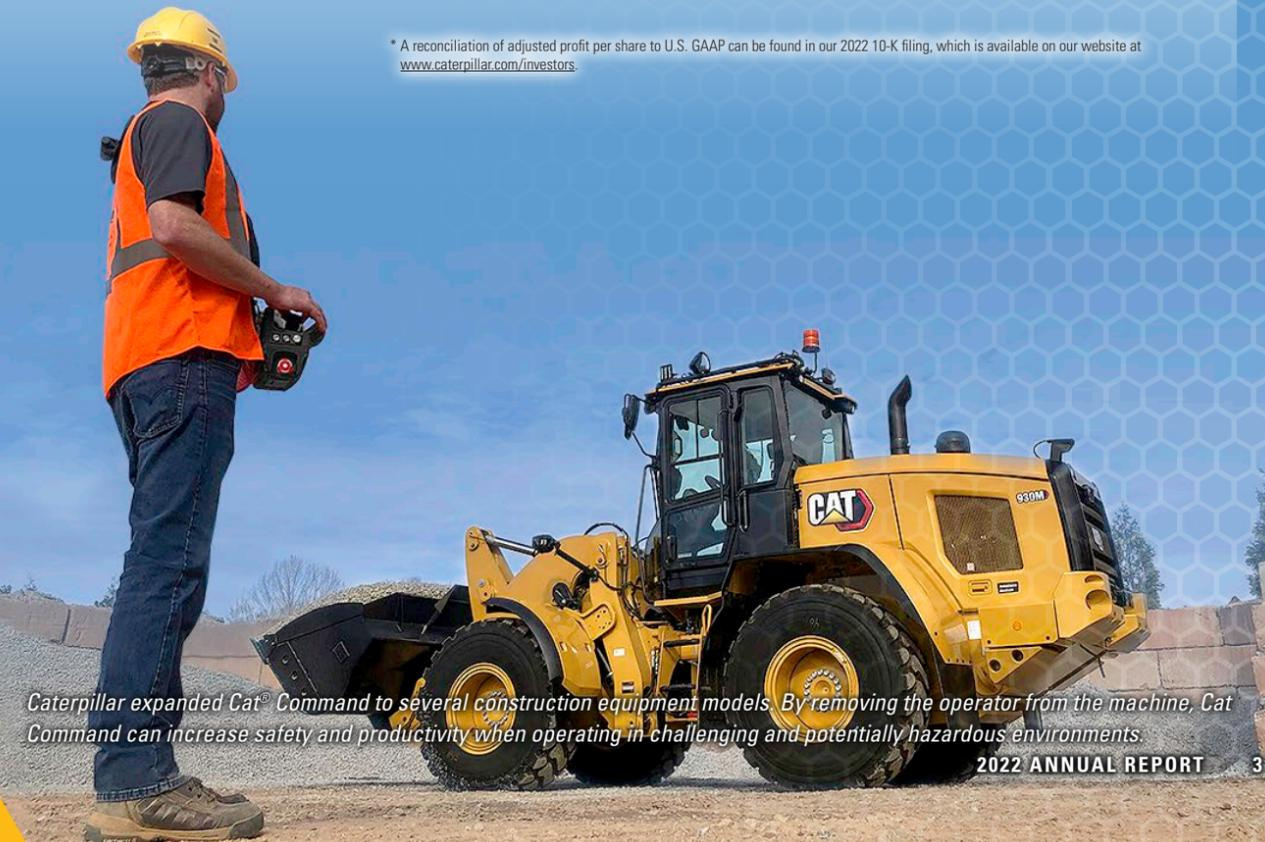
Caterpillar expanded Cat® Command to several construction equipment models. By removing the operator from the machine, Cat Command can increase safety and productivity when operating in challenging and potentially hazardous environments.
