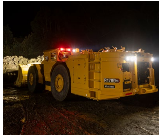
Cat R1700 XE battery electric, zero-exhaust emissions underground mining Load Haul Dump (LHD) with onboard battery
