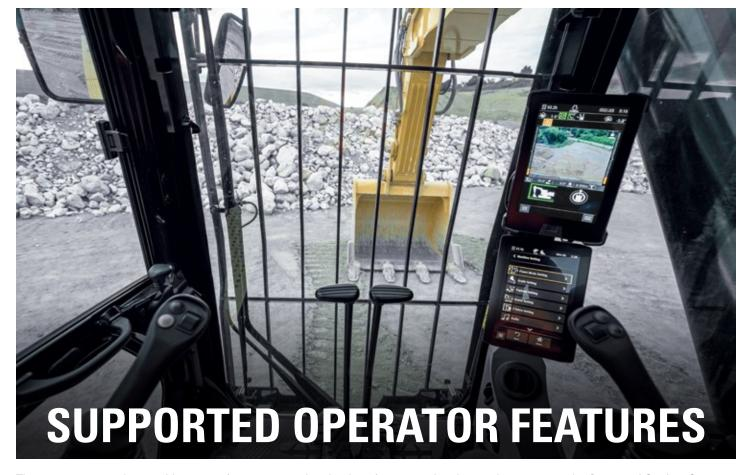
The operator can select a wide range of excavator and technology features using the touch screens on the Command Station. Some features are not available on all excavator models or configurations. Consult your Cat dealer for details.
