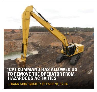
SAIIA, an industrial/heavy civil contractor in northern Alabama, is using three Cat Command Stations around an ash pond site. The materials around these ponds can be unpredictable, especially during rainy conditions.
