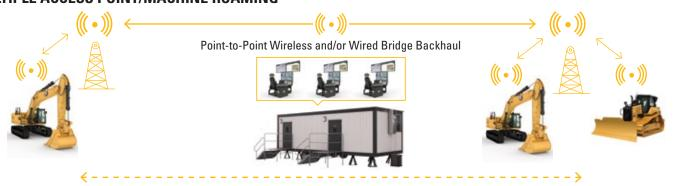
Machine Can Roam Between Multiple Access Points
