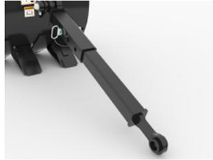
The G108 uses the same fixing point as the current thumbs. No weld or paint job is needed to install.
