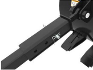
Stiff link can be manually adjusted in three positions by repositioning the pin position. No special tools are required.
