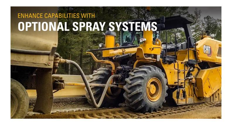
Computerized water and emulsion additive systems accurately monitor application rates for precise distribution. Using the touch screen display in the cab, operators can turn spray nozzles on or off to customize spraying width and easily set up the spray systems for the delivery of liquid additives according to specifications:
