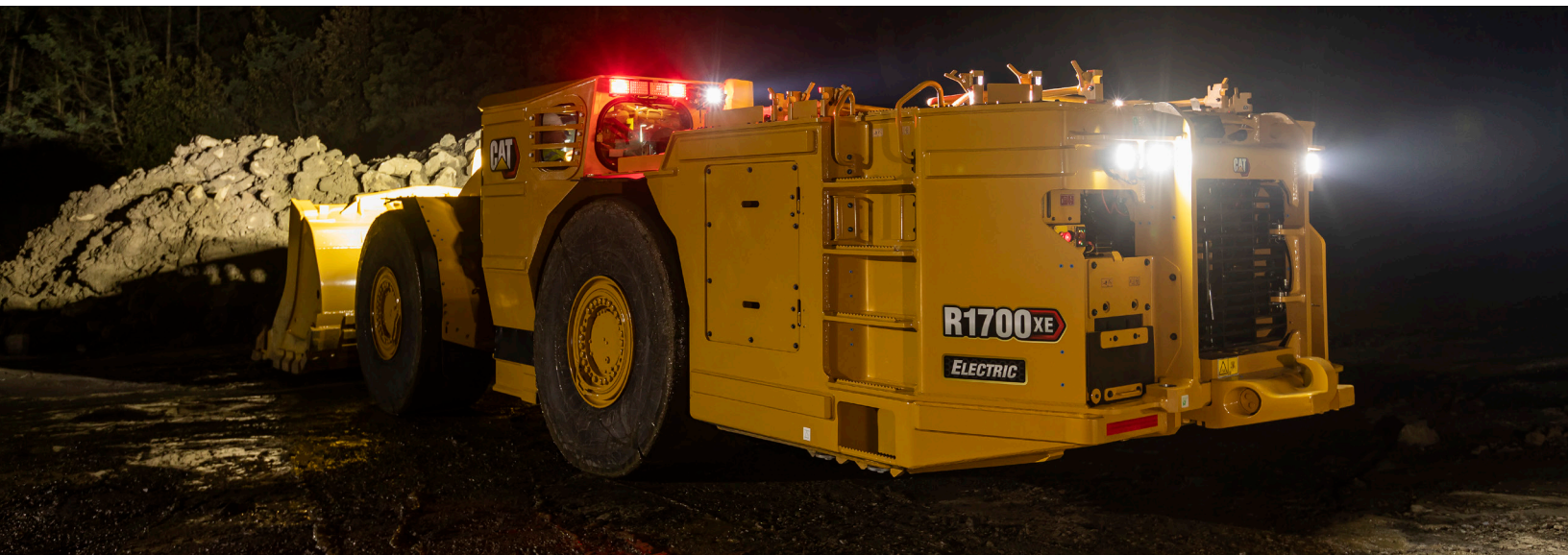
Cat® R1700 XE battery electric, zero exhaust emissions underground mining Load Haul Dump (LHD) with onboard battery
