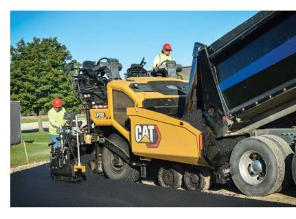
of less than 18 ft.-6 in. and width of 8 ft.-6 in, these 13- to 15-ton pavers can be transported without special permits. The front-loading angle of 17 degrees and high bumper clearance simplify unloading and loading without the need for additional blocking.
