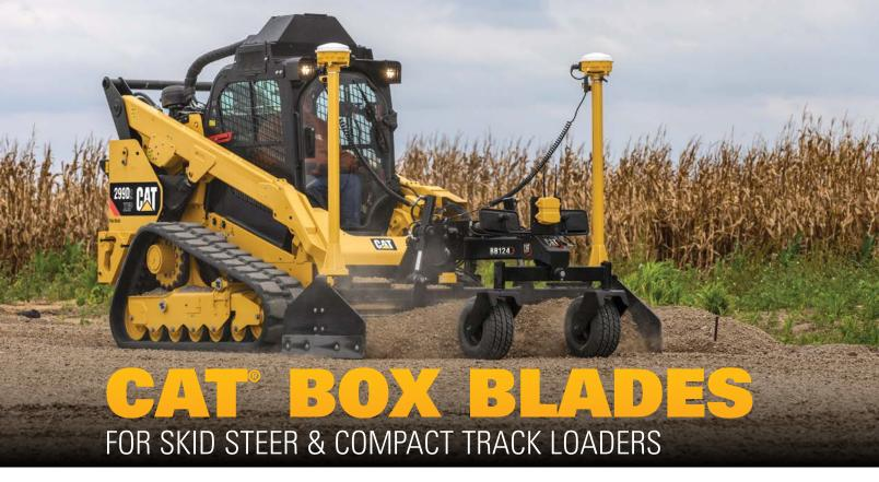
Designed for grading and leveling, Cat<sup>®</sup> Box Blades are ideal for large commercial properties, housing pads, roadways and parking lots. The BB121 (7 ft) and BB124 (8 ft) attachments operate both manually and automatically with the use of laser or GPS grading systems. The following features will help you handle your agency's work faster:
