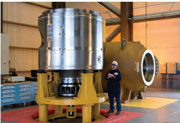
**Figure 5-5.** Bundle (Module) and centerbody.
