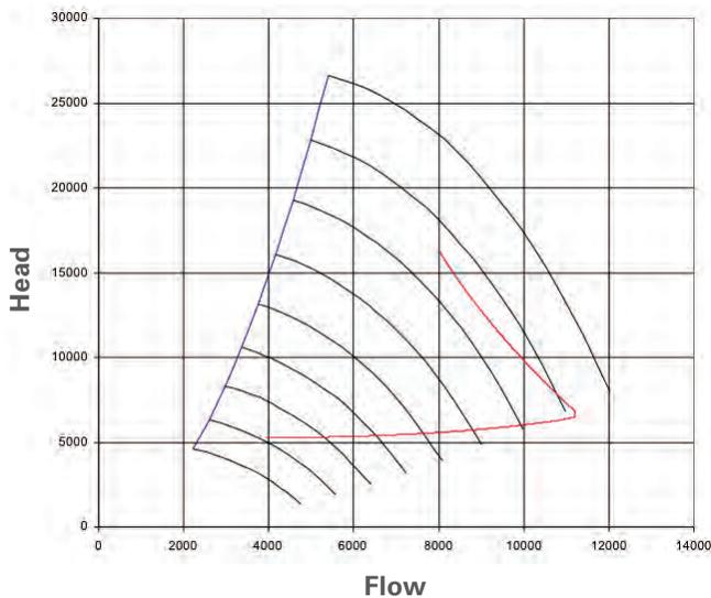
**Figure 6-13.** Typical operating points, if transient conditions are considered, in this case due to a fast engine acceleration from 50% to 100% load (Kurz et al [13]).
