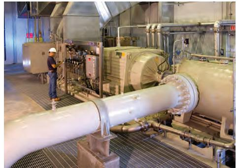
**Figure 7-5.** Electric-motor drive package: constant-speed motor driving the compressor via a variable-speed gearbox.
