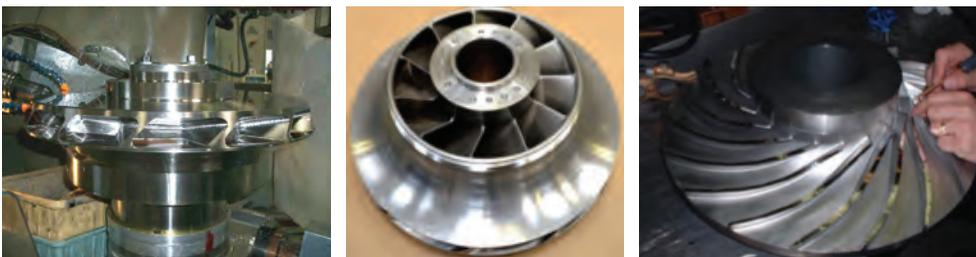
**Figure 5-7.** Impeller manufacturing methods: (left) machined, (center) cast, (right) machined with brazed shroud.
