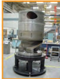
**Completed rotor diaphragm assembly**
