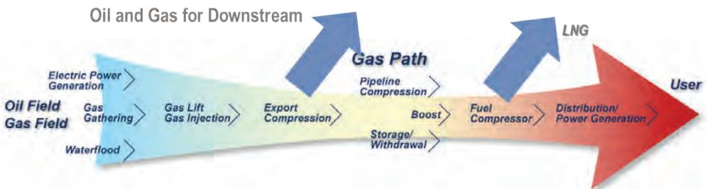
**Figure 8-1.** Natural gas movement from the well to the user.
