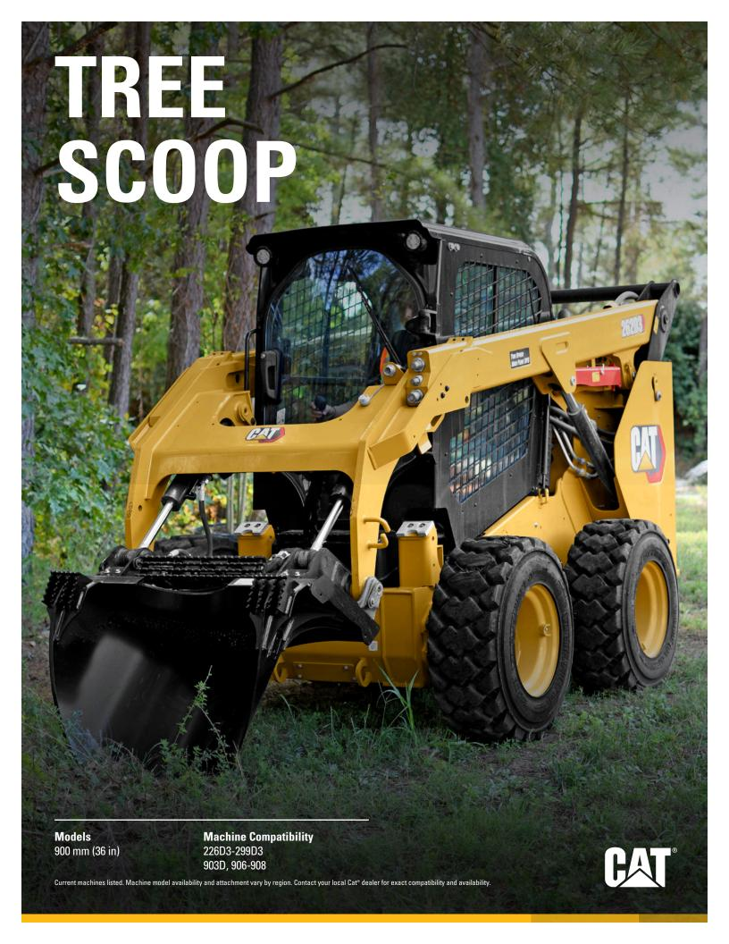
The Cat® tree scoop is designed for handling shrubs and small trees at nursery sites and in landscaping applications. The spade profile can dig and scoop up to a 901 mm (36 in) diameter, allowing easy transport or transplant of trees and much more.
