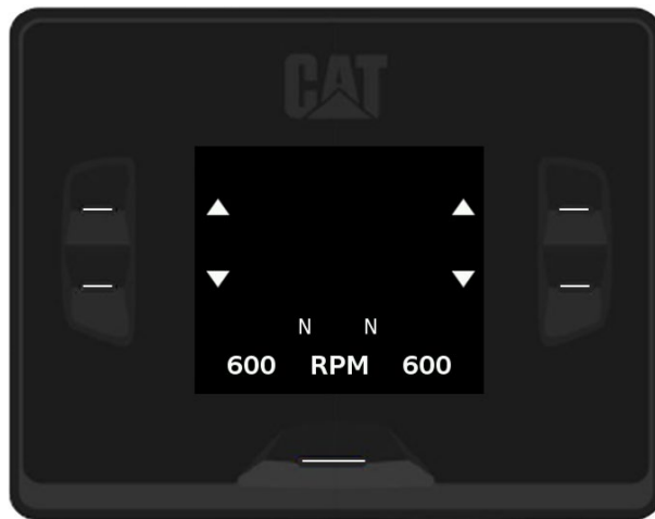
Figure 78: Transfer to backup panel, low idle and neutral gear
