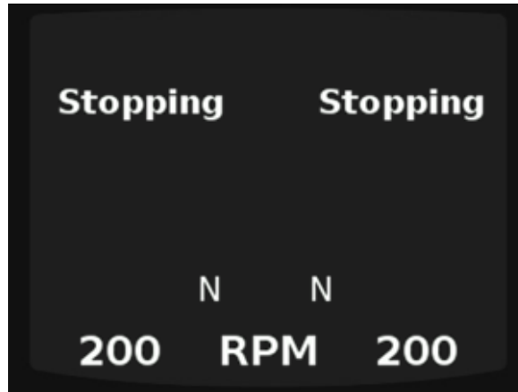
Figure 87: Remote Start/Stop Stopping
