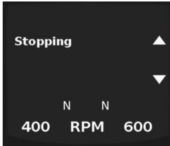
Figure 89: PORT Remote Start/Stop Button Pressed Again (engines running)
