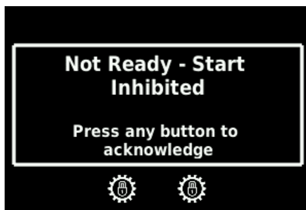
Figure 82: Second press of the start button when the engines are not ready
