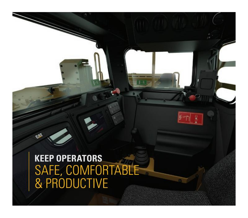
The R1600H features an operator station that is ergonomically designed for total machine control in a comfortable, productive and safe environment. All controls, levers, switches and gauges are positioned to maximize productivity and minimize operator fatigue.
