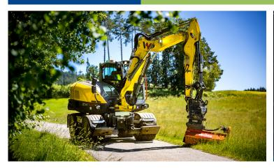
The EW100 reaches a maximum speed of 40 km/h – perfect for fast job site changes, while the powerful drive hydraulics and working power enables the compact machine to complete work typically undertaken by a 14-ton mobile excavator.
