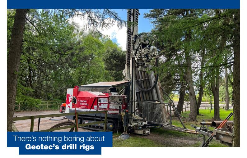
Drilling into the earth may seem like a simple process, but in reality there are many different techniques available to meet a broad range of application requirements. Modern vertical drill rigs are used for near-surface geothermal energy extraction, geotechnical engineering, mining and well construction, using techniques including dry drilling with casing, cable percussion drilling with casing, suction drilling and core drilling plus drilling with endless or hollow stem augers.
