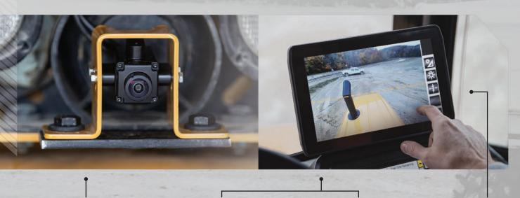
A high-definition camera placed at the back of the machine allows operators to have rear visibility. An in-cab mounted display gives the operators a high-resolution view — allowing them to notice small, important details.
