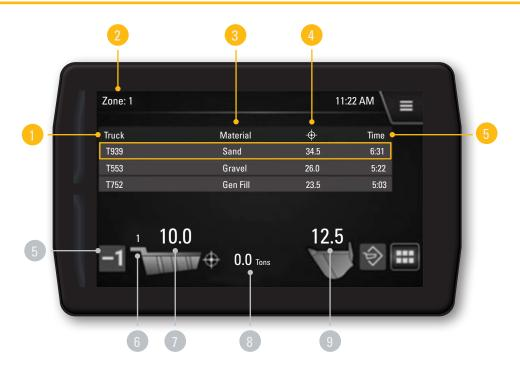
Dispatch for Loading works with Advanced Payload to provide loader operators with all the details needed to load the correct truck with the right amount of material.
