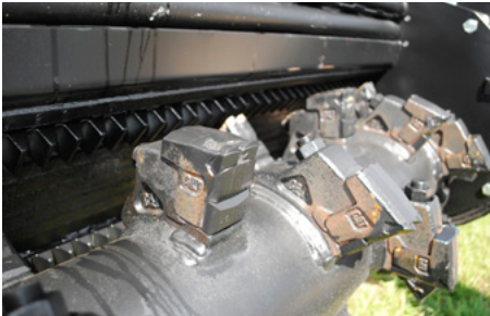
Single bolt carbide tooth retention
