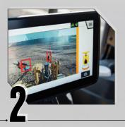
A high-definition, touchscreen display provides the operator with additional views around the machine and engages with the operator when a person is detected behind the machine.
