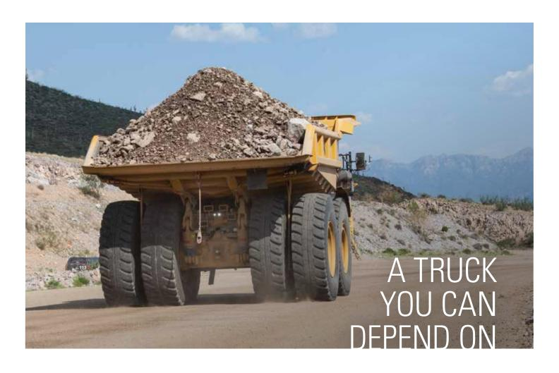
The 789 has been a dependable performer on mine sites for decades, delivering high availability, reliability and reduced costs that come with long life — from the engine and powertrain to the components, brakes and frame. Component life is further enhanced thanks to the standard rear-axle continuous filtration feature. Cleaner oil helps promote longer lubrication that leads to longer life.
