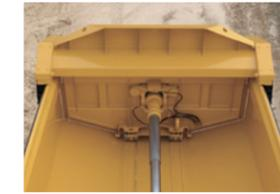
**ARTICULATED DUMP TRUCK BULK EJECTOR**
