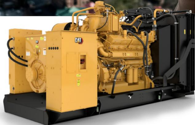
By using elevated jacket water temperatures, specialized exhaust valves and stainless steel aftercooler cores, these generator sets help combat the presence of contaminants in waste-generated gas to ensure durability and reduce operating costs.
