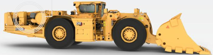
Integral ROPS and FOPS cab, resiliently mounted to the frame
