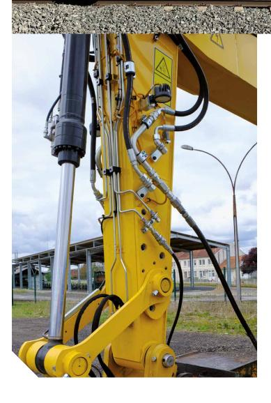
The M323F is factory built with all hydraulics required for railway dedicated tools. Standard auxiliary hydraulics, including high pressure and quick coupler lines and circuits, allow easy attachment changes without the need to add additional lines to your machine.
