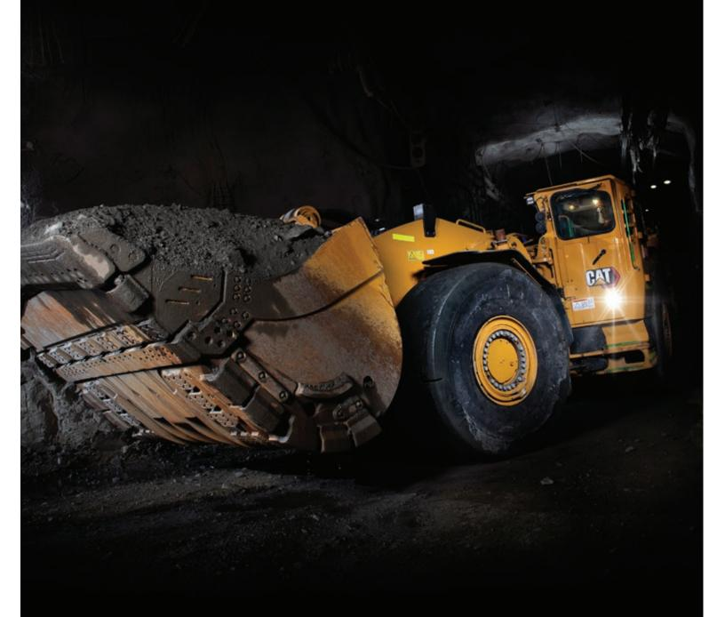
Rated Payload: Rated Power – peak: Rated Power – nominal: Operating Weight: 15 000 kg / 33,069 lb 250 kW / 335 hp 220 kW / 295 hp 48 743 kg / 107,460 lb
