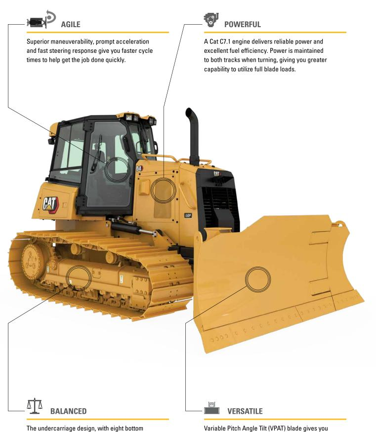
rollers and two carrier rollers, is optimized for smooth finish grading and a better ride, even at faster grading speeds.
