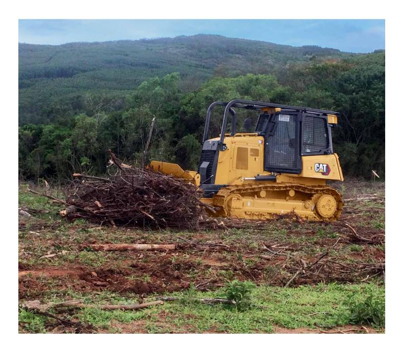
If you work in severe environments, add protection for your dozer and operator with optional features like a heavy-duty cab, sweeps and window/door screens. Specialized guarding protects machine components. Hydraulic demand fan and turbine air precleaner help handle high debris situations. LED lights add visibility. Ask your Cat dealer about the factory options that are right for your applications.
