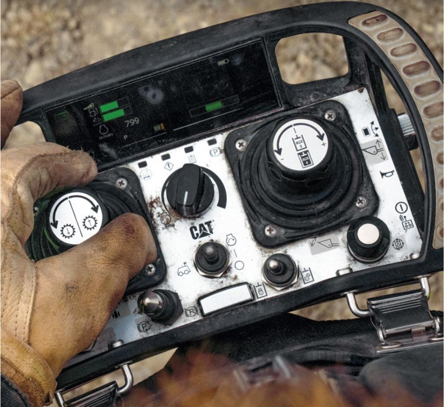
Cat Command Console and Cat Command Station controls are fully integrated with the wheel loader's electronic and hydraulic systems.
