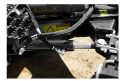
Manual or hydraulic angling up to 20 degrees right or left of center. Hydraulic angling option allows the operator to control the power box rake angle from the operator compartment.
