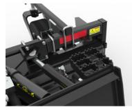
Wide access step with grating and large profile serrations provides better traction for entering and exiting the cab.
