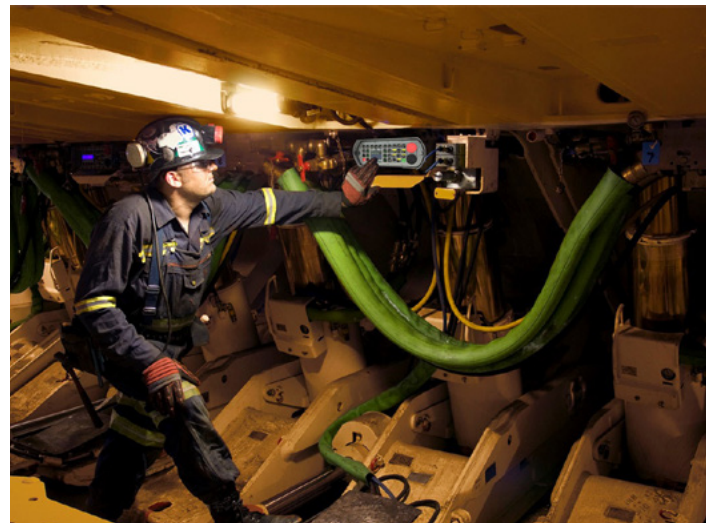
PMC controllers are protected by stainless steel housings to withstand harshest conditions underground
