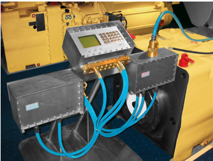
Configuration of PMC-D and PMC-V connected to a CST drive
