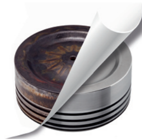
MaK piston crown before and after refurbishment.
