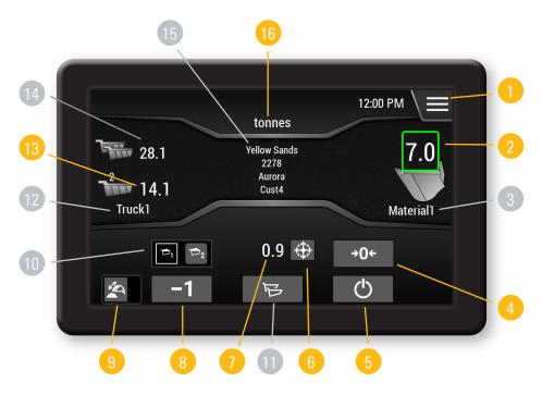
Advanced Payload Display Shown (Display Can Vary By Machine Model)
