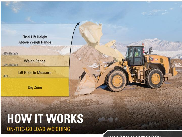
The Cat Payload system calculates material weight on-the-go by using data from sensors that measure bucket position and hydraulic pressure (certain features require the Advanced Payload system).
