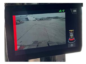
When a person is in the off-display zone, the system will provide red or yellow on-screen indicator bars based on proximity to the machine.
