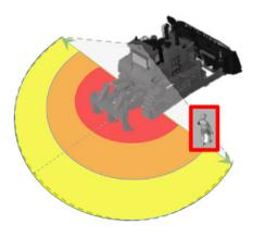
The system detects personnel in a wider field of view than is shown on the display. Visual alerts indicate a person in the off-display zones.
