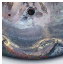
An example of increased crown temperatures leading to severe lacquering on the underside of the piston, thermal overload, material burn off and potential piston failure.
