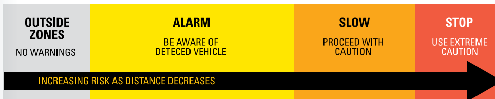
Each zone is site configurable (number, size, alarm patterns, alarm suppression options, etc.)
