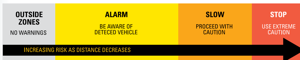
Each zone is site configurable (number, size, alarm patterns, alarm suppression options, etc.)
