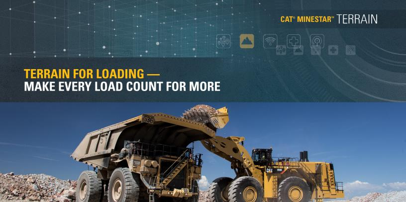
Mine site output depends on efficient loading and hauling. Cat® MineStar™ Terrain for loading makes those operations more productive while providing accurate feedback to key personnel. It shows operators the type of material and the exact volume that is being loaded into trucks and crushers. Real-time feedback on payloads and design plan progress helps managers track materials and plan future operations.
