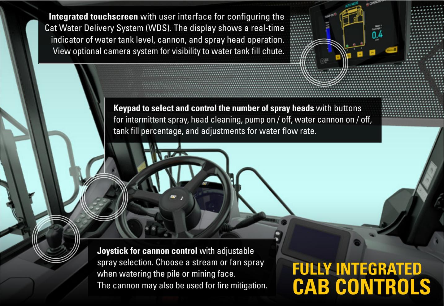
**Integrated touchscreen** with user interface for configuring the Cat Water Delivery System (WDS). The display shows a real-time indicator of water tank level, cannon, and spray head operation. View optional camera system for visibility to water tank fill chute.
