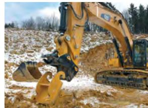
**Hex CW Couplers:** Excavators, Wheeled Excavators and Material Handlers
