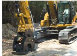
**Compactor Plates:** Backhoe Loaders, Excavators and Wheeled Excavators
