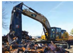
**Scrap Shears:** Compact Track Loaders, Multi-Terrain loaders, Excavators, Skid Steer Loaders, Wheeled Excavators and Material Handlers
