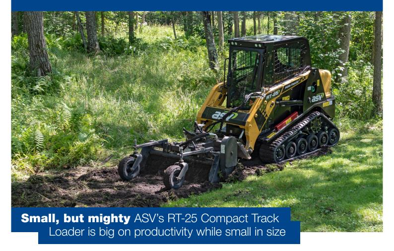
Size matters, but probably not in the way you think. When it comes to compact track loaders, as the name suggests small does have its advantages, but power is still important. The ASV RT-25 is the world's most compact track loader and, thanks to the Perkins® 403J-17T, 25-horsepower, three-cylinder diesel engine with turbocharger, it's also powerful.
