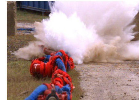
Destructive testing conducted with a designed failure at 22,500 psi on up to 4" iron utilizing SPM™ FSR
