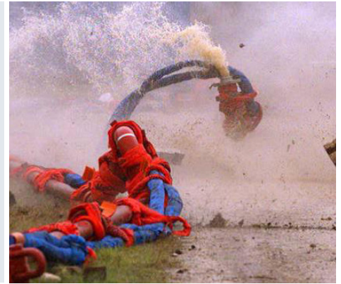
Right: Testing validated SPM™ FSR and proved ability to reduce the danger area around high pressure hydraulic fracturing operations.
