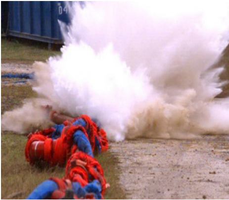
Left: Destructive testing conducted with a designed failure at 22,500 psi on up to 4" iron utilizing SPM™ FSR
