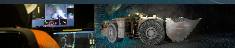
Command for underground enables remote operation of load-haul-dump machines, providing immediate productivity and efficiency gains and improving safety by removing operators from hazardous environments.
