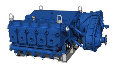
The SPM® QEM 3000 Frac Pump from SPM Oil & Gas answers the industry's demand for longer hours of operation and increasing rod load. This specially designed pump allows continuous duty pressure pumping operation at 275,000 lbf rod load 100% of the time.
