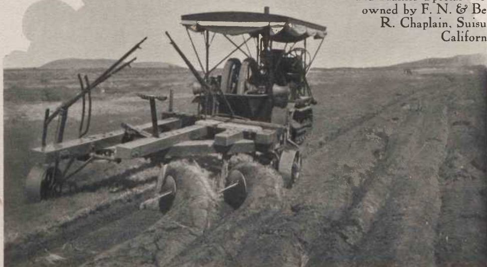
In Virgin Soil, pastured since reclaiming. Pulling 2, 24 inch Plows, at a depth of 12 inches
